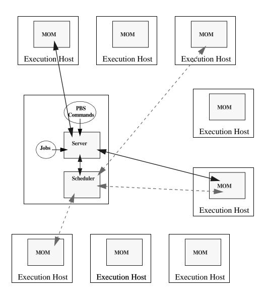
This diagram illustrates multi-node cluster configurations wherein the Scheduler and Server communicate with the MOMs on the compute nodes. Jobs are submitted to the Server, scheduled for execution by the Scheduler, and then transferred to a MOM when its time to be run. MOM periodically sends status information back to the Server, and answers resource requests from the Scheduler.
